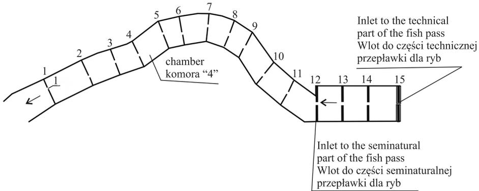
Fig. 3. Diagram of fish passes along with the location of hydrometric vertical [Szustakowska 2015]
