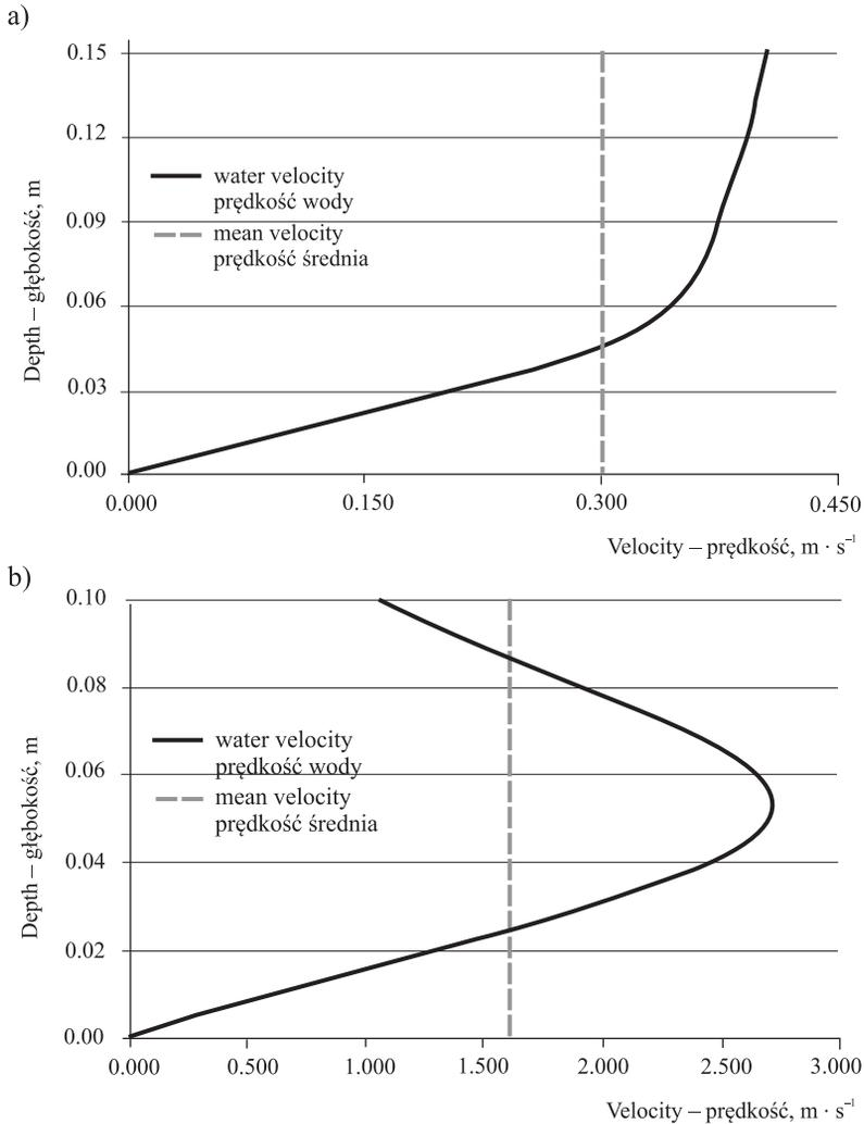
Fig. 7. Water velocity and average water velocity: a) outlet of the technical section of the fish pass, b) inlet to the technical section of the fish pass
