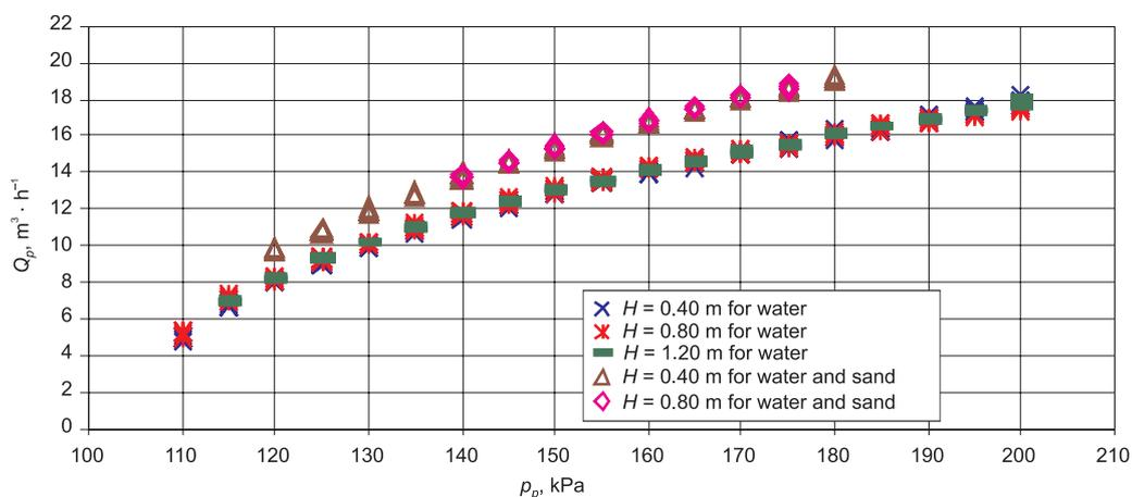
**Fig. 3.** Air flow rate  $Q_p$  in the air lift pump vs. air pressure  $p_p$  and water-sand mix lifting height  $H$
