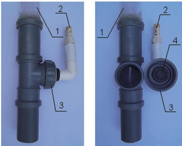
**Fig. 2.** Construction of the mixer with perforated rubber diaphragm – type PM 50:
