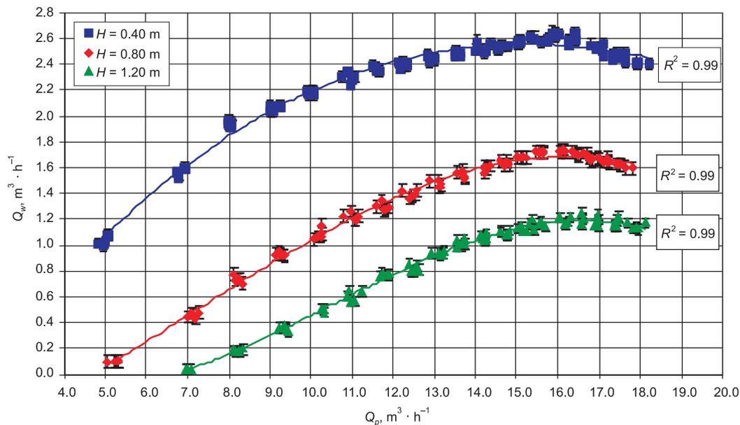
**Fig. 4.** Water flow rate  $Q_w$  vs. air flow rate  $Q_p$
