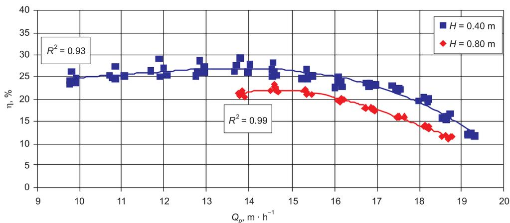
**Fig. 6.** Efficiency  $\eta$  of the air lift pump depending on the air flow rate  $Q_p$  – for water and sand
