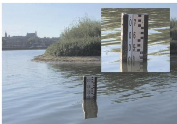
**Fig. 1.** Warsaw gauging station on August 29, 2015 on the river Vistula. Water level – 42 cm
