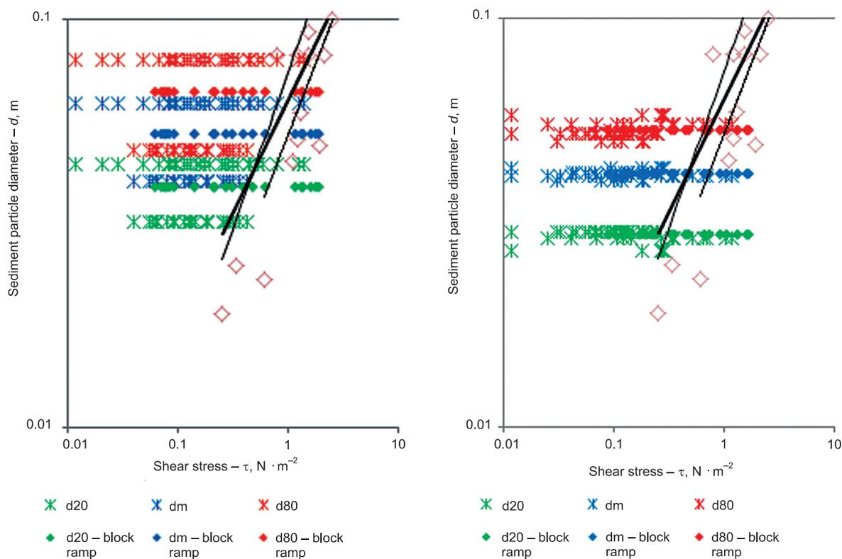
**Fig. 9.** Graph showing the threshold shear stress for the bed-load transport at 3b (left) and 4a (right) measurement series (Radecki-Pawlik 2014)
