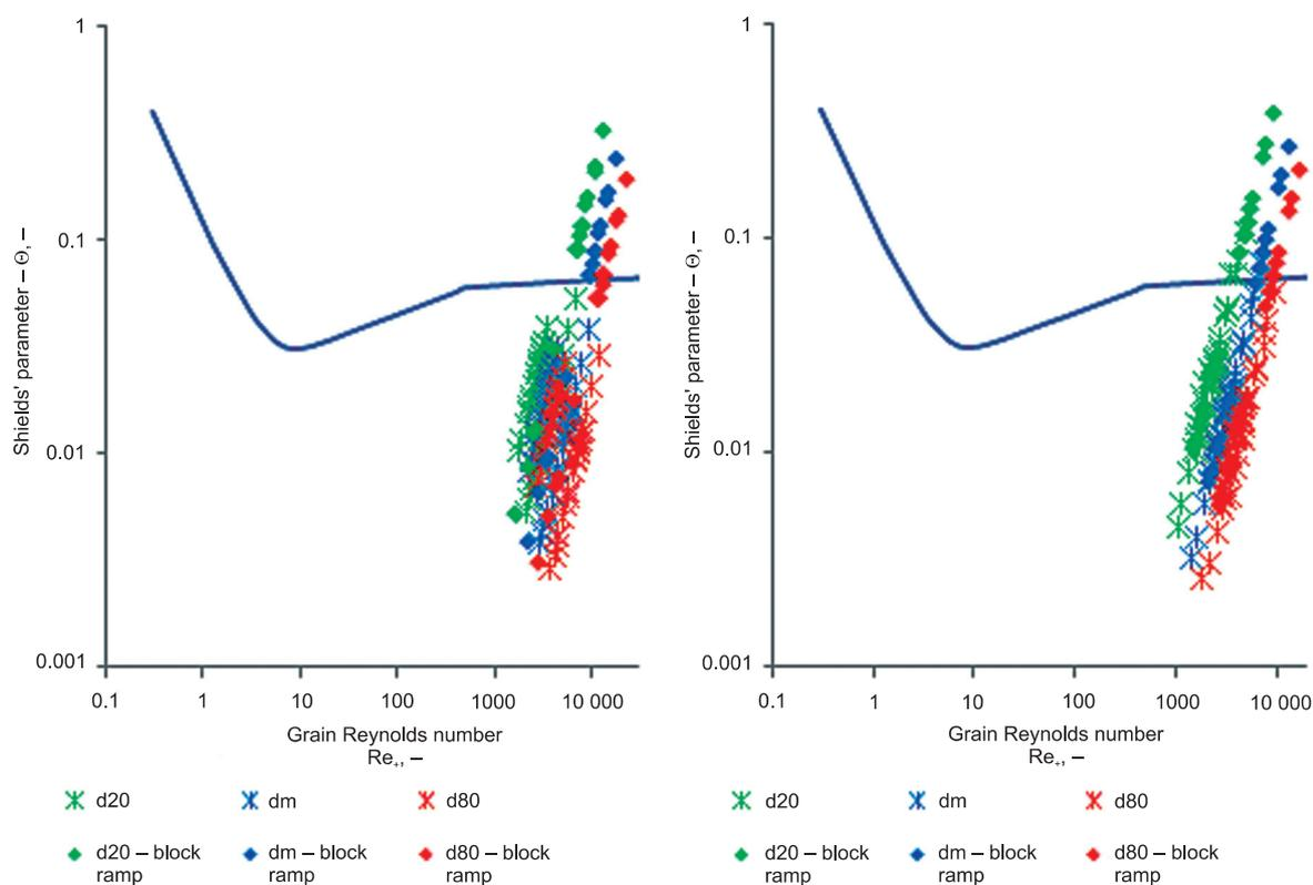
**Fig. 10.** Shields' diagram for bed-load transport at measurement points of the 3b (left) and the 4a (right) series (Shields 1936)
