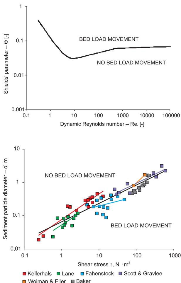
**Fig. 2.** Shields' diagram (Shields 1936) (a) and the graph showing the beginning of bed load transport movement depending on shear stress (b) (Radecki-Pawlik 2014)
