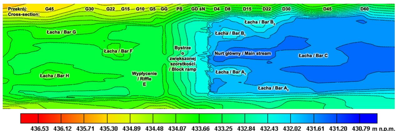
Fig. 4. Riverbed morphology observed during the measurement series 1a
