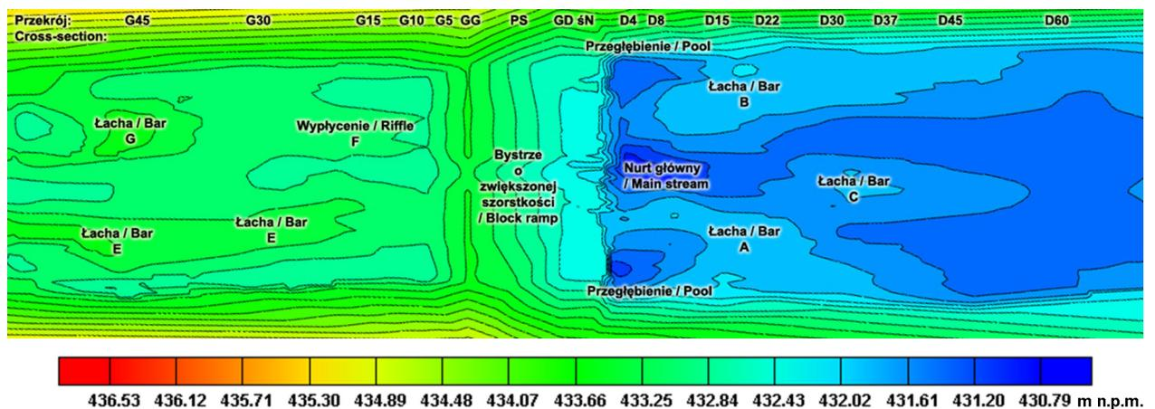
Fig. 8. Riverbed morphology observed during the 4a–4b measurement series
