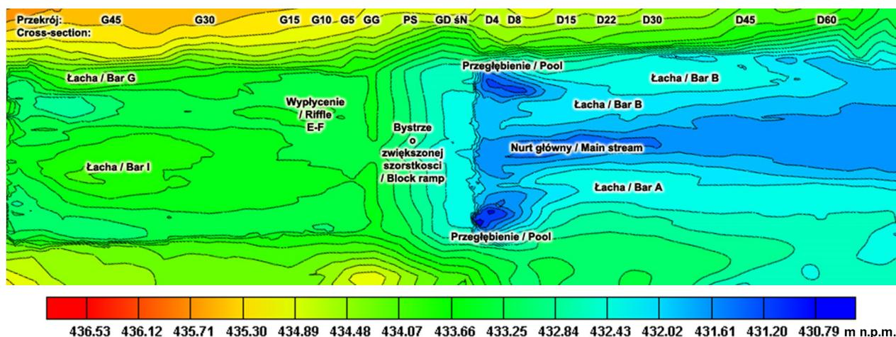
Fig. 6. Riverbed morphology observed during the 2a–2b measurement series
