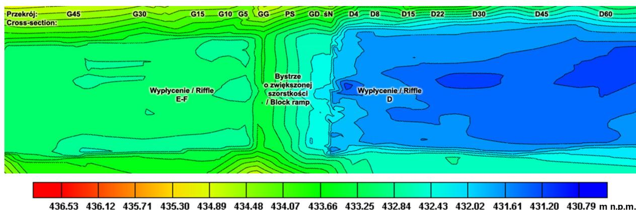
Fig. 7. Riverbed morphology observed during the 3a–3b measurement series
