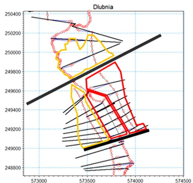
Fig. 3. Schematization of the Zesławice reservoir's bowl
