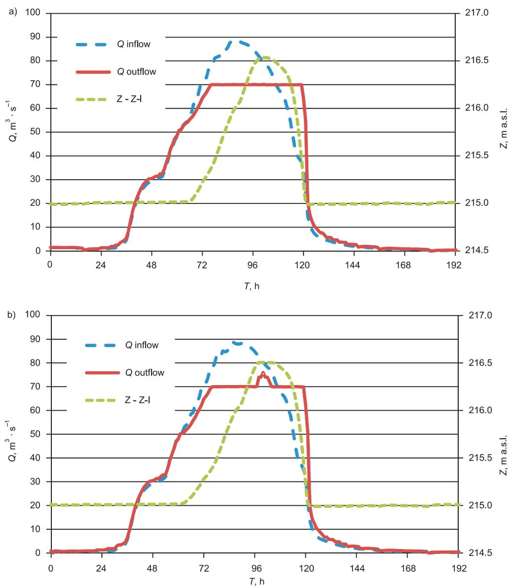
**Fig. 7.** The results of  $Q_{5\%}$  flood wave simulation through the Zesławice reservoir according to: a) variant VI, b) variant VII
