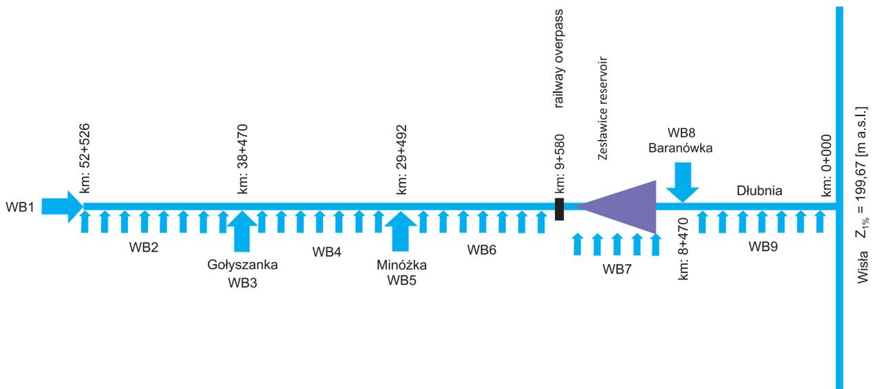
**Fig. 5.** Scheme of boundary conditions of the Dłubnia River model
