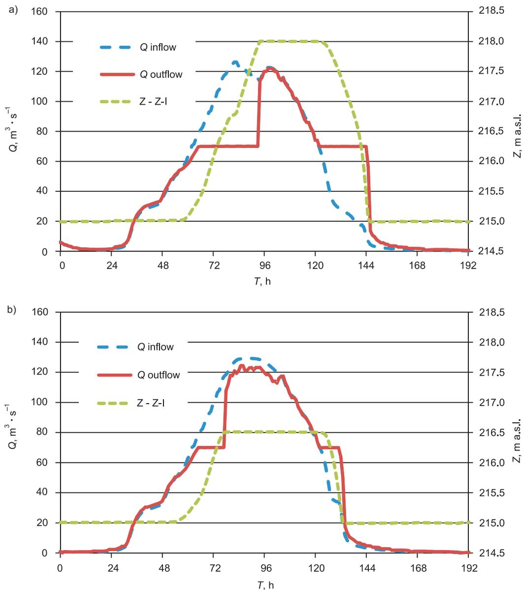
**Fig. 6.** The results of  $Q_{1\%}$  flood wave simulation through the Zesławice reservoir according to: a) variant VI, b) variant VII
