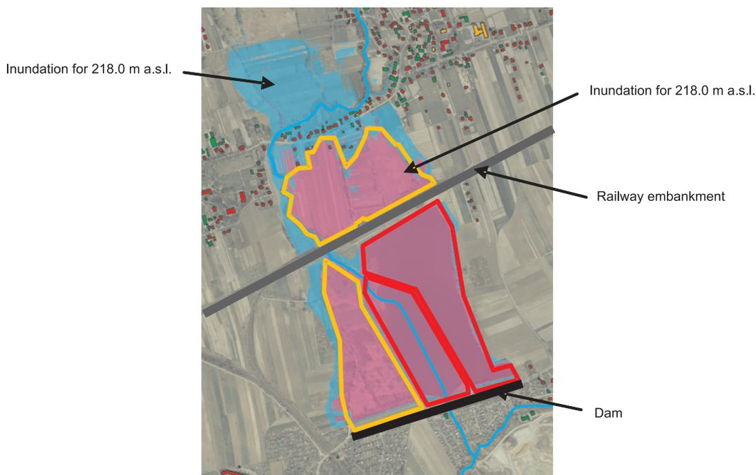
**Fig. 2.** Spatial arrangement of the reservoir elements
