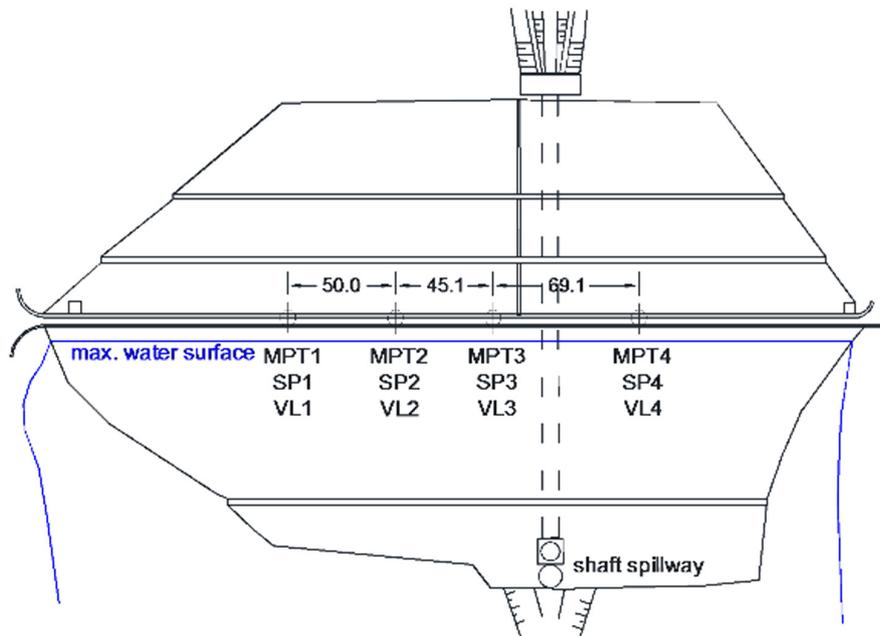
**Fig. 5.** Karolinka VD – situation of mounted probes EIS (Pařílková et al. 2016b)
