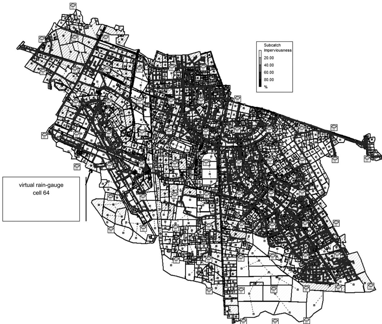
**Fig. 4.** Sub-catchments, channels and virtual rain-gauges in the investigated catchment, shown in the SWMM model
