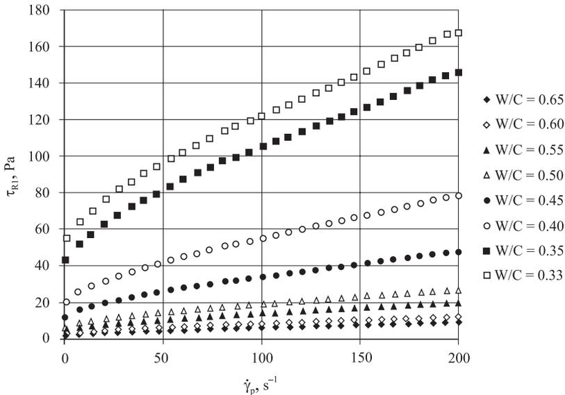
Fig. 3. Pseudo-curves of flow of cement pastes.
