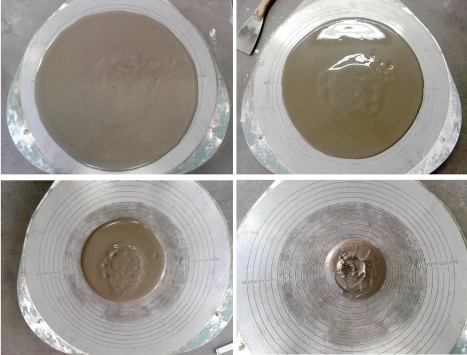
Fig. 1. Slump tests of cement pastes, W/C = 0.65, 0.60, 0.45, 0.35
