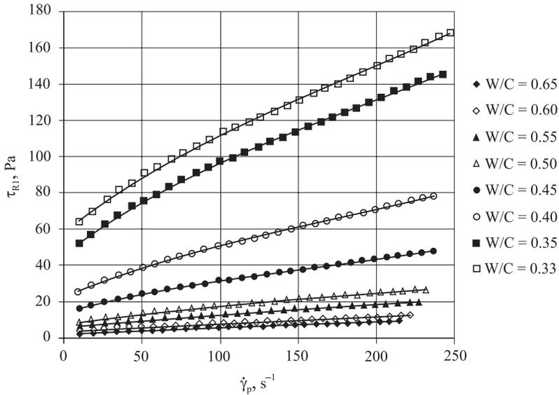
Fig. 4. Actual curves of flow of cement pastes.
