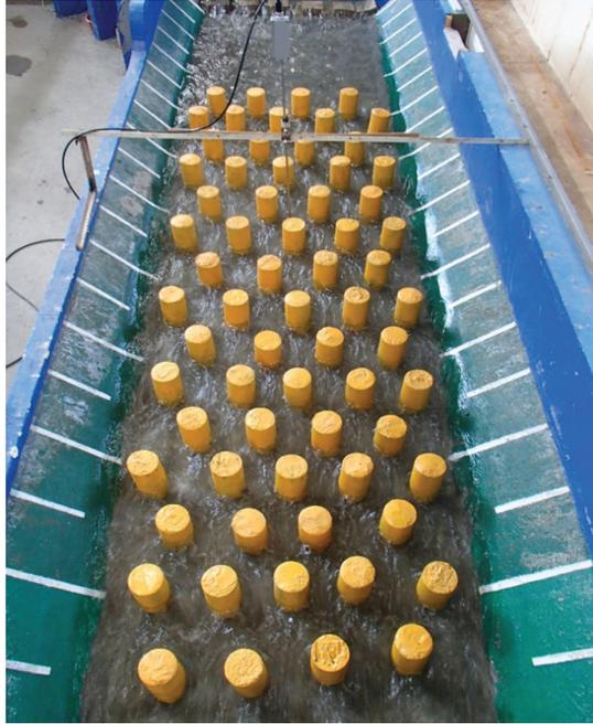
Fig. 2. Diagram showing the spacing of cylindrical stones in fish pass
