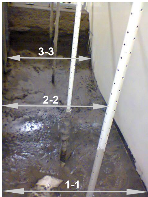
Fig. 4. Cross-section through the model embankment 1 (P1–P6 – water level measuring pipes)
