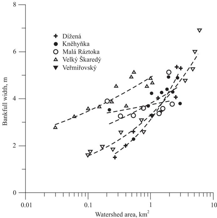
Fig. 3. Plot of the dependence of the watershed area and the bankfull width of studied channels
