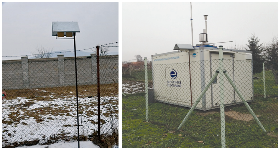
Fig. 1. Meteorological booth with filtering plates
