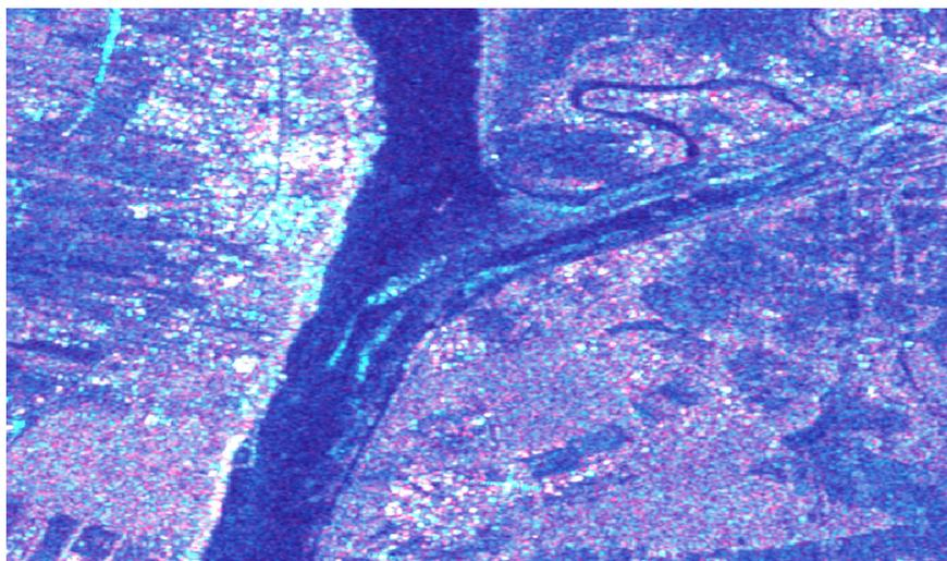
**Fig. 5.** Mouth of the Bug river to Dębe reservoir shown at color composite image recorded by Sentinel-1 satellite on February 14, 2017 where: R- Amplitude\_VH, G- Amplitude\_VV, B –  $\log_{10}(\text{Amplitude\_VV})$  – at Bug river it is visible contact between mobile ice and static ice and white field of ice jam upstream
