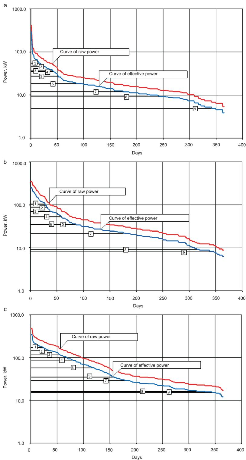
**Fig. 3.** Power curves: a – 1969 dry year, b – 1971 – medium year, c – 1974 – wet year, 1 –  $3.0SQ$ , 2 –  $2.5SQ$ , 3 –  $2.0SQ$ , 4 –  $1.5SQ$ , 5 –  $SSQ$ , 6 –  $SQ$ , 7 –  $Q_{50\%}$ , 8 –  $NTQ$ , 9 –  $Q_{95\%}$
