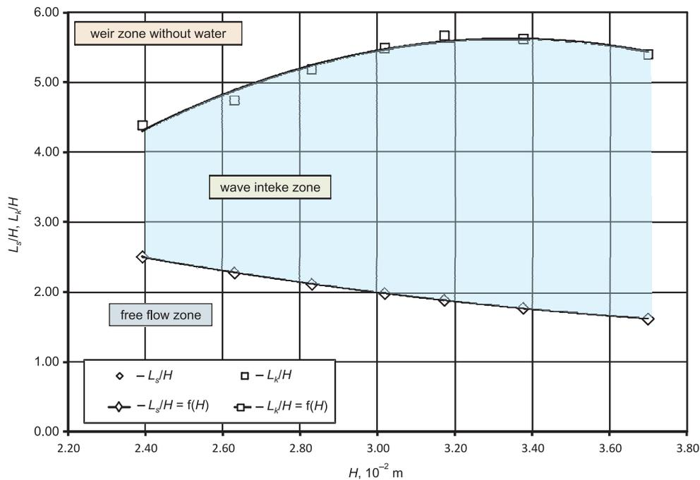
**Fig. 5.** Ranges of stream zones on the permeable sill
