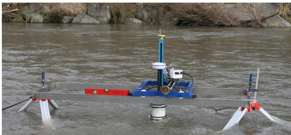
**Fig. 2.** Measuring station in the main channel, the Skawa River at kilometre 19 + 293,  $Q = 17.6 \text{ m}^3 \cdot \text{s}^{-1}$ , Series 1
