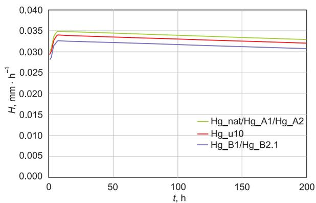
**Fig. 7.** Comparison between hydrographs of the component of groundwater feed  $H_g$  simulated in the model for different location variants of urbanized areas
