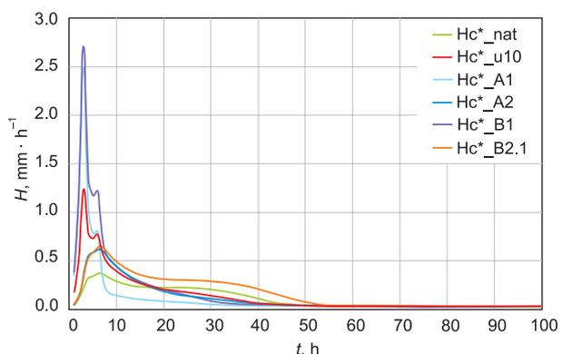
**Fig. 5.** Comparison between hydrographs of the component describing total feed into the riverbed  $H_{c^*}$  simulated in the model for different location variants of urbanized areas
