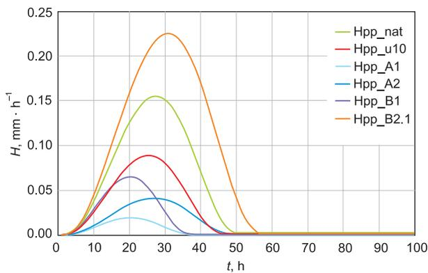
**Fig. 6.** Comparison between hydrographs of the component of subsurface feed  $H_{pp}$  simulated in the model for different location variants of urbanized areas
