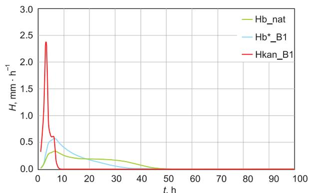
**Fig. 4.** Change of the hydrograph of direct runoff component as a result of additional feeding of the riverbed with the runoff of rainwater sewage B1 type areas –  $H_{kan\_B1}$
