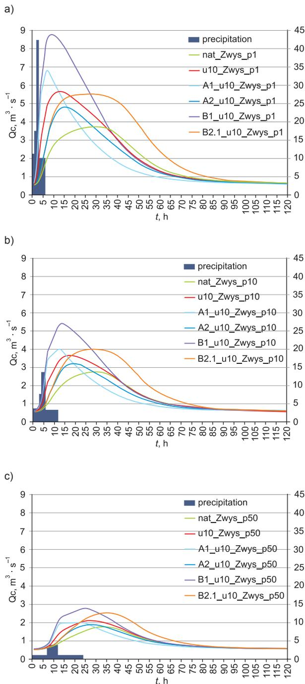
**Fig. 2.** Formation of total runoff from catchment urbanized in 10% with various types of areas, in the conditions of high waterlogging, and precipitation with the probability of overrun amounting to a) 1%, b) 10%, c) 50%; symbols as in table 1
