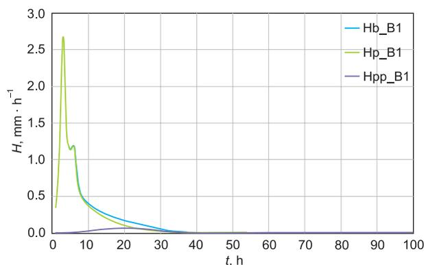
**Fig. 3.** Hydrograph of feeding the river channel with direct runoff, and its components, simulated for urbanized catchments in areas of B1 type
