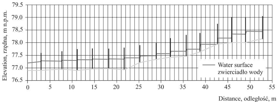
Fig. 5. Longitudinal profile of the fish pass together with the number of chambers and the water surface level in the chambers
