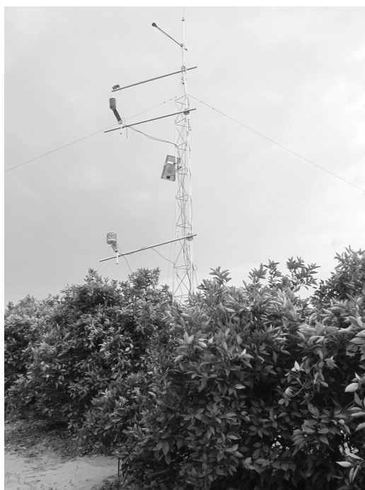
Fig. 2. Site of the study plot (orange grove of 80 ha): equipments for measuring the necessary parameters to determinate the actual evapotranspiration, using the Bowen ratio method
