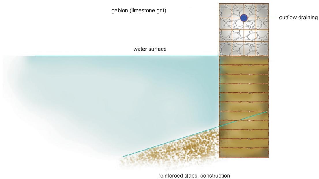
**Fig. 9.** The form of strengthening of the bank of a filter pond (edited by Ewelina Widelska)
