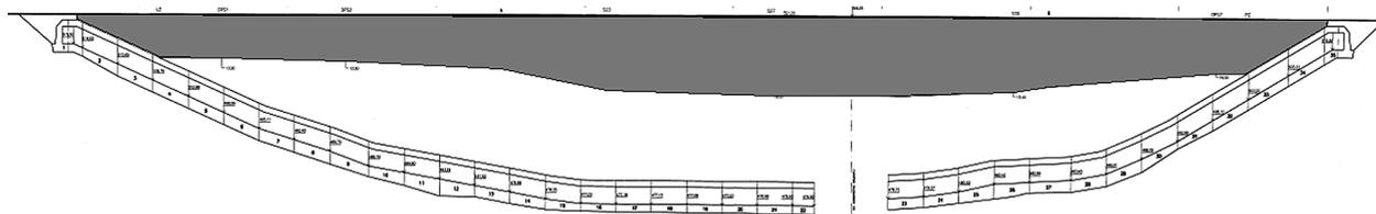
**Fig. 2.** A longitudinal section through the earth-fill dam of the Karolinka VD with a newly constructed wall (Jareš and Krejčí 2014)
