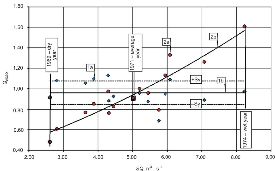
**Fig. 5.** Dimensionless values of installation flows: 1a – measurement points  $Q_i/SQ$ , 1b – mean value  $Q_i/SQ$ , 2a – measurement points  $Q_i/SSQ$ , 2b – regression curve  $Q_i/SSQ$
