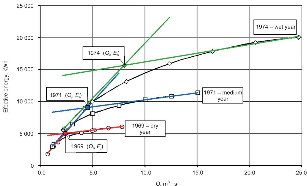
**Fig. 4.** Effective power as a function of the specified discharge
