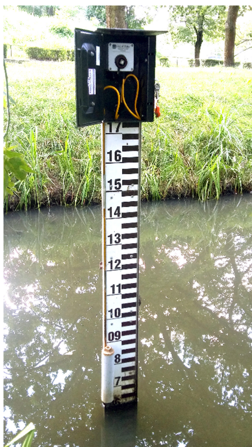
Fig. 2. Gauge Station upstream of the Staw Wyścigi (Pond), optical turbidity sensor with data recorder and gauge staff (photo by A. Krajewski)
