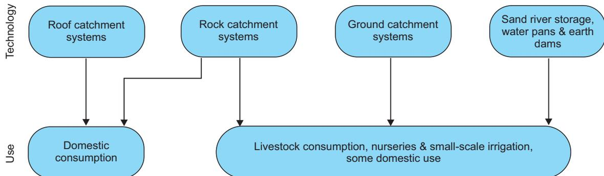
**Fig. 3.** Implementation system of rainwater harvesting systems and uses (source: Kimani et al., 2015)
