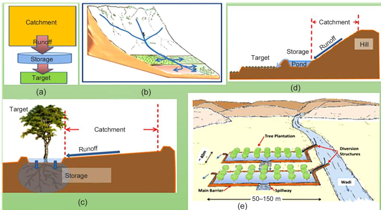
**Fig. 1.** (a) The operation steps of rainwater harvesting; (b) Schematic diagram of macro catchment system; (c) Micro catchment system; (d) Schematic diagram of a macro catchment system with a pond for intermediate storage of runoff; (e) Floodwater diversion under climate change (source: Prinz, 2013)
