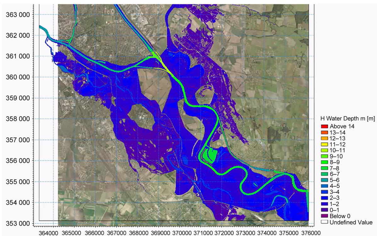
**Fig. 4.** Dam break simulation at Łany near Wrocław city for a flood with exceedance probability  $p = 1\%$  (source: own elaboration)
