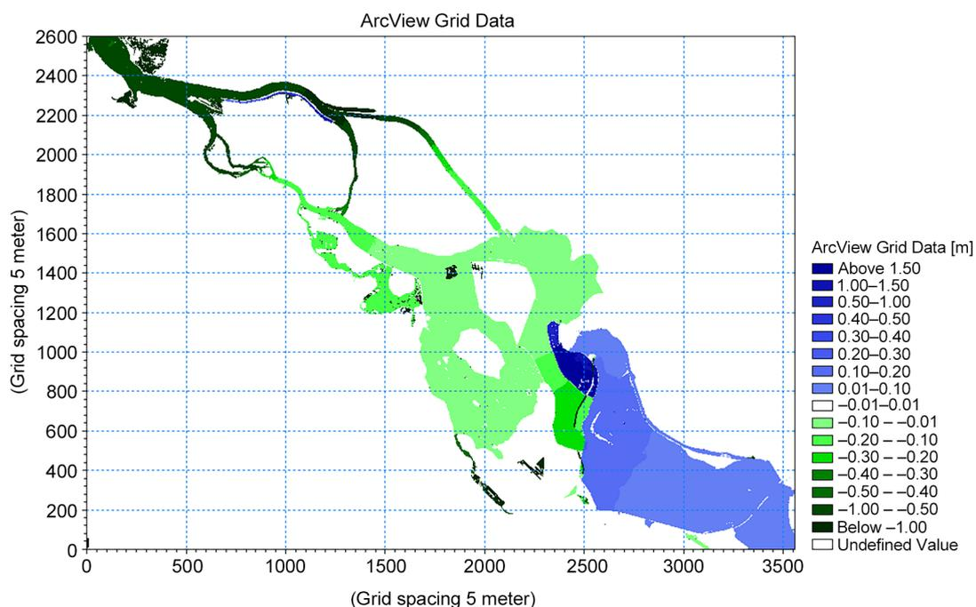
**Fig. 3.** Change of the water level due to the modernization of the Wrocław Water Node (for the design discharge) (source: own elaboration)
