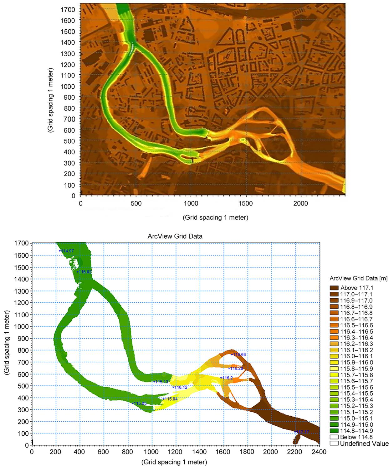
**Fig. 2.** 2D model of the Wrocław City Centre Hydrosystem: bathymetry of the 2D model (upper part) and the calculated water level for the 2010 flood (with the measured water levels) (source: own elaboration)
