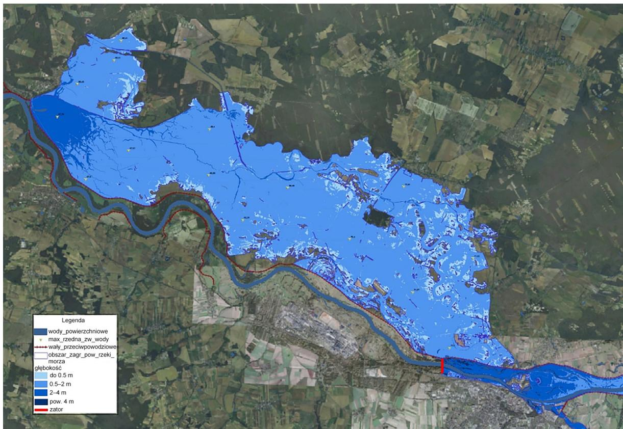
Fig. 5. Modelling of flooding caused by ice jams near the city of Głogów (source: own elaboration)
