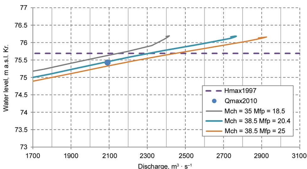
**Fig. 6.** Calculated upper part of the rating curve for the Głogów cross-section (roughness factor for the main channel –  $M_{ch}$ , for floodplain –  $M_{fp}$ , observed maximum water level in 1997 –  $H_{max}$ , recorded maximum discharge during the flood in 2010 –  $Q_{max}$ ) (source: own elaboration)
