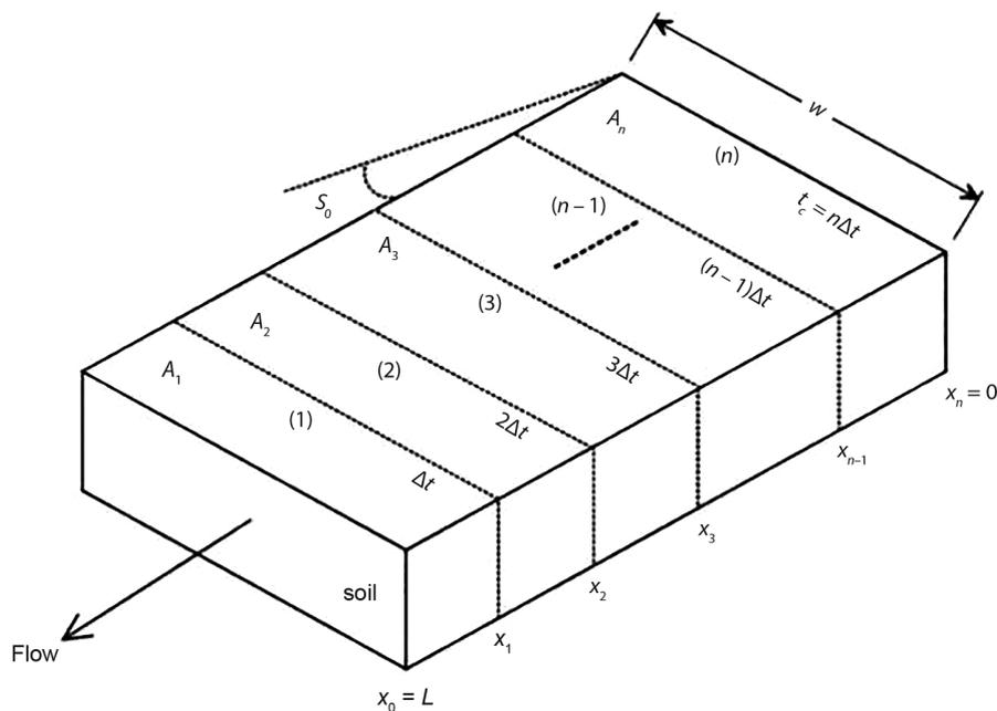
Fig. 2. Subsurface isochrone curve of a soil layer (source: after Fariborzi et al., 2019)
