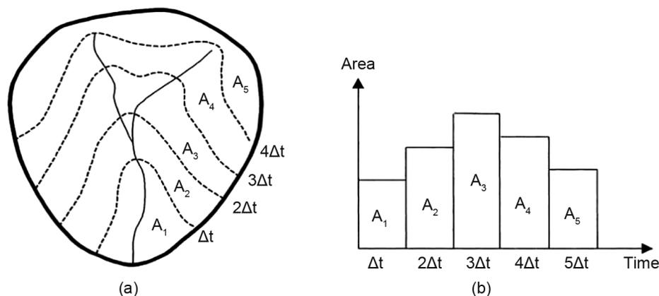
**Fig. 1.** (a) Isochrones of a basin; (b) time-area histogram (source: after Saghafian et al., 2002)
