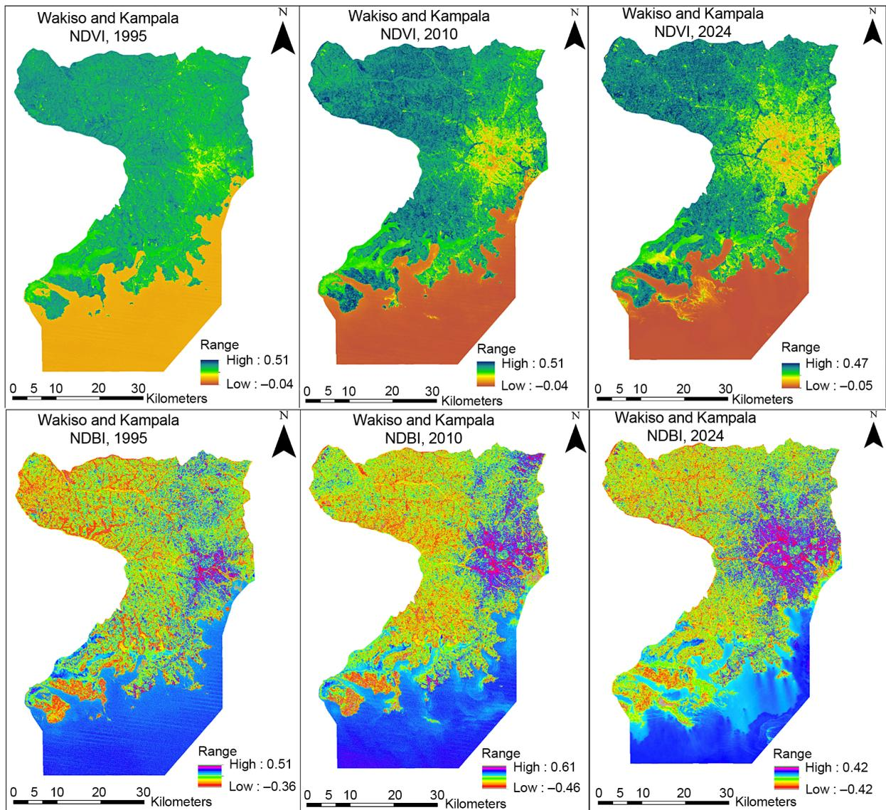
**Fig. 6.** LULC conversion patterns based on NDVI and NDBI (source: generated by Authors' using Landsat 5 imagery for 1995 and 2010, and Landsat 8 imagery for 2024)
