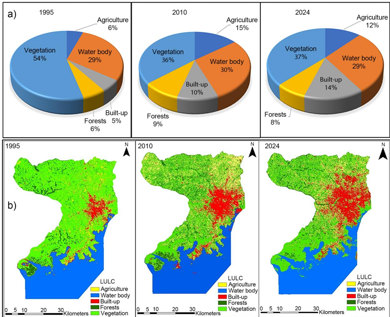
**Fig. 2.** State of Land Use/Land Cover Wakiso and Kampala districts in Uganda for the periods, 1995, 2010, and 2024 (source: generated by Authors using Landsat 5 (1995 and 2010) and Landsat 8 (2024) satellite imagery, classified using supervised classification in ArcGIS 10.4)
