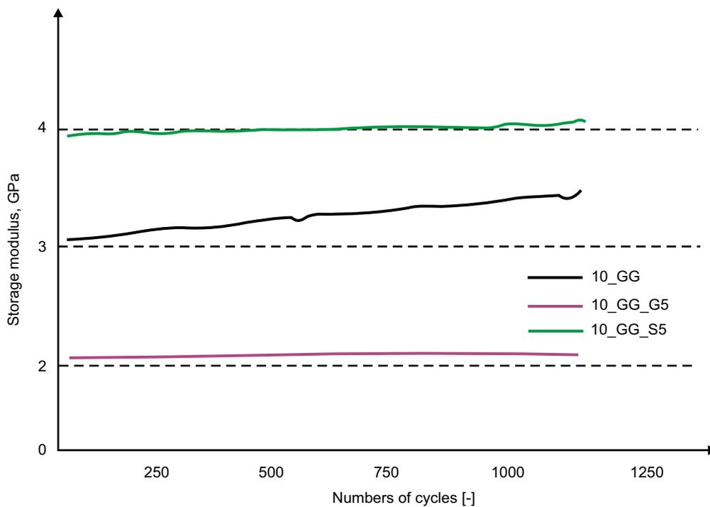
**Fig. 6.** Storage modulus curve for the hydrogels tested (source: Authors' own elaboration)
