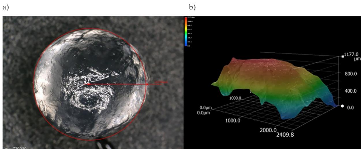
**Fig. 2.** Microscopic photograph of a) a hydrogel sphere with b) surface analysis (source: photo by Authors)
