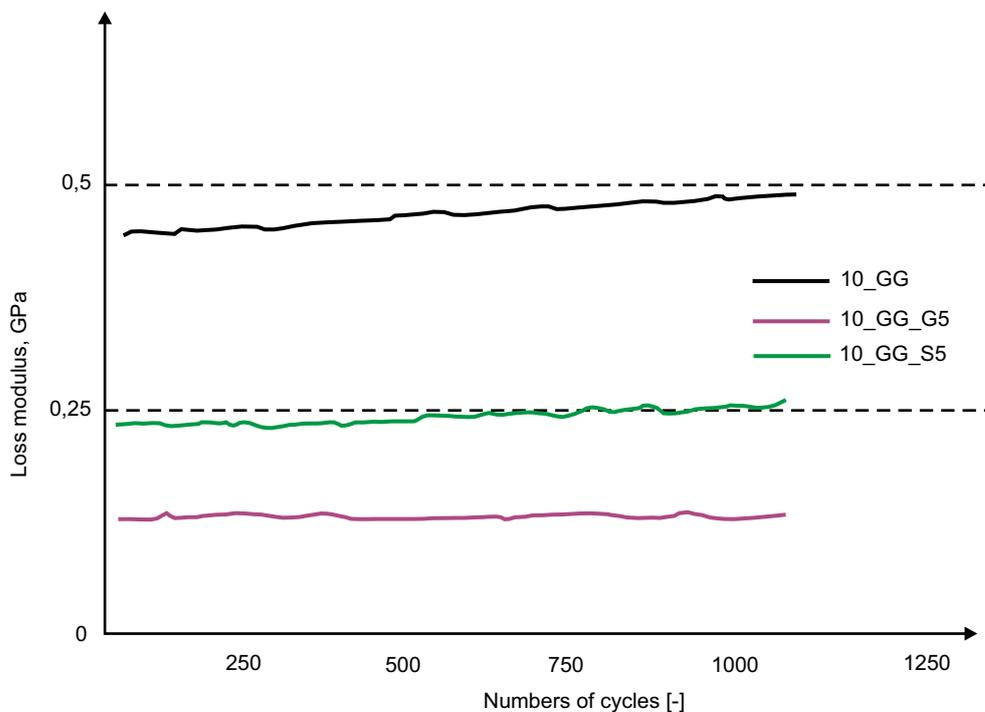
**Fig. 7.** Loss modulus curve for the hydrogels tested (source: Authors' own elaboration)
