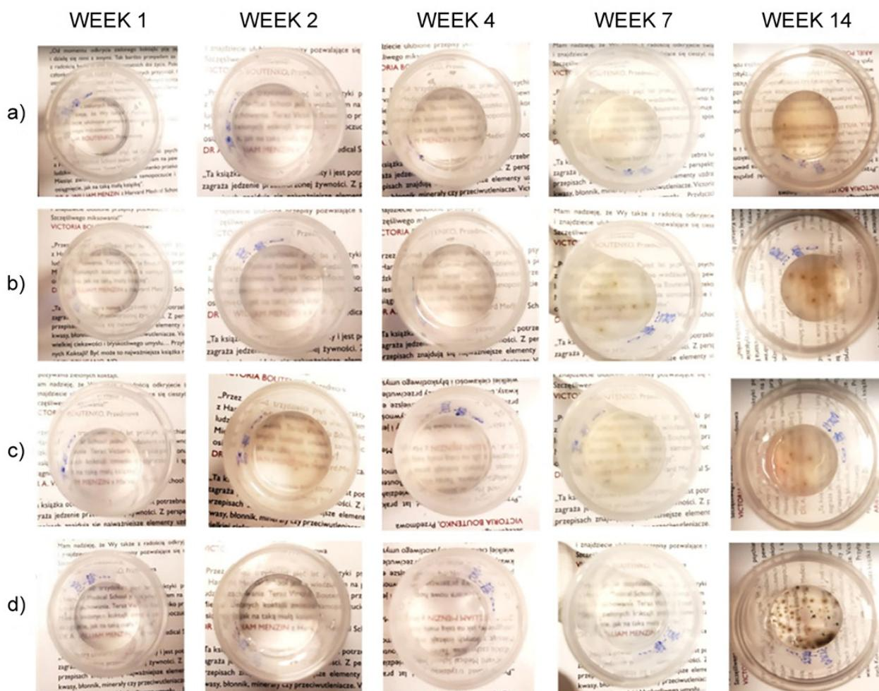
**Fig. 12.** Comparison of changes in hydrogel appearance over time for: a) 10\_GG, b) 10\_GG\_S5, c) 10\_GG\_S3\_G2, d) 10\_GG\_G5 (source: photo by Authors)
