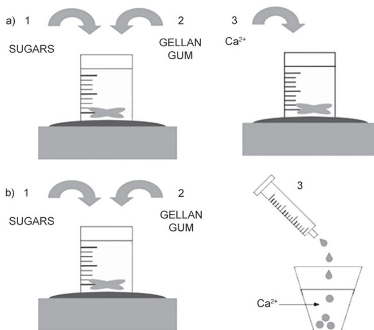
**Fig. 1.** Schematics of substrate fabrication: a) in continuous form and b) in spherical form (source: Authors' own elaboration)
