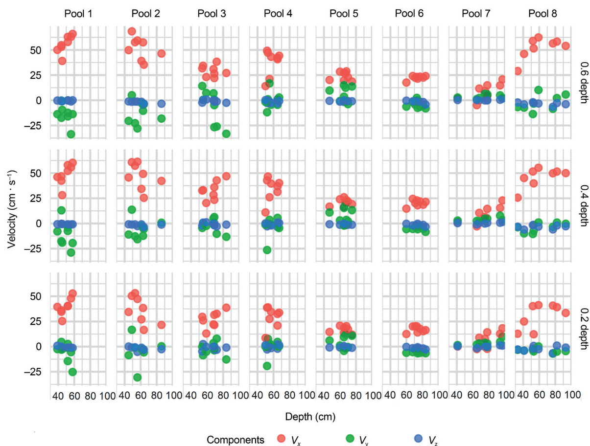
Fig. 1. Distribution of flow velocity components in eight investigated pool units (Pool 1 – Pool 8). Streamwise ( V_x ), transverse ( V_y ), and vertical ( V_z ) velocities are shown for three relative depths ( z/h = 0.2, 0.4, 0.6 ; h – local flow depth) (Source: Authors' own elaboration)
