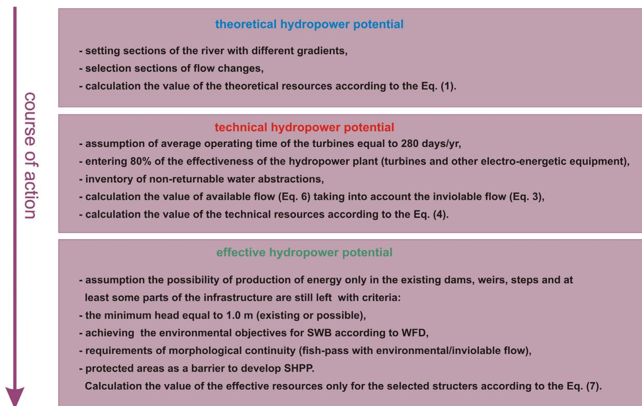
**Fig. 2.** Course of action for effective potential of hydropower assessment in Upper Vistula water region (Operacz, 2017 modified)
