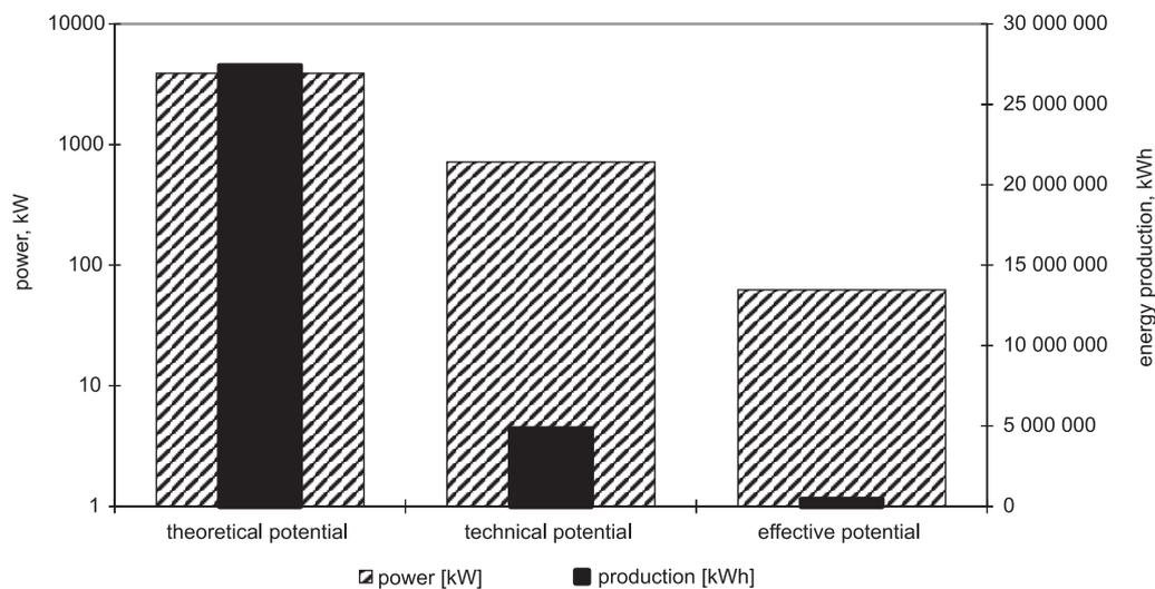
**Fig. 5.** Comparison of power and energy production estimated by theoretical, technical and effective potential of hydropower
