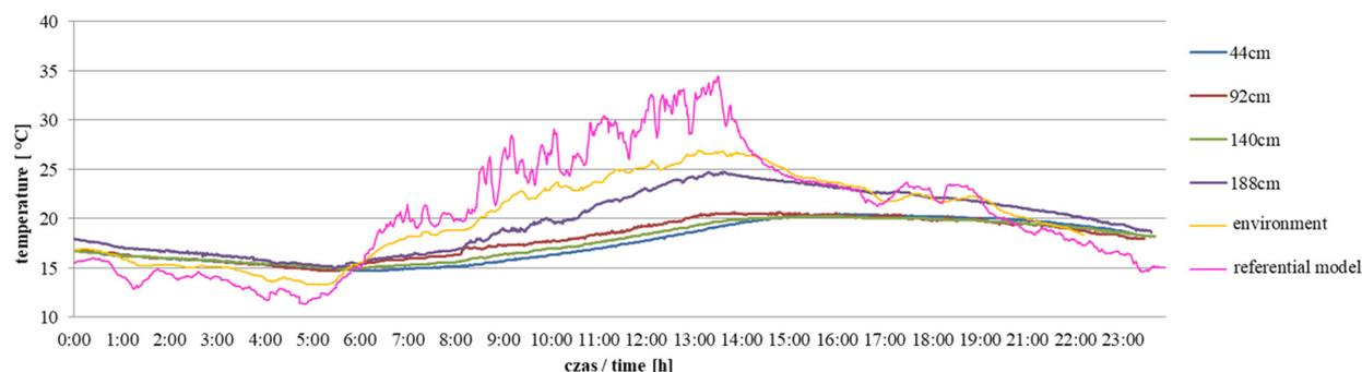
**Fig. 2.** Distribution of temperatures within the substrate on 28 May 2016
