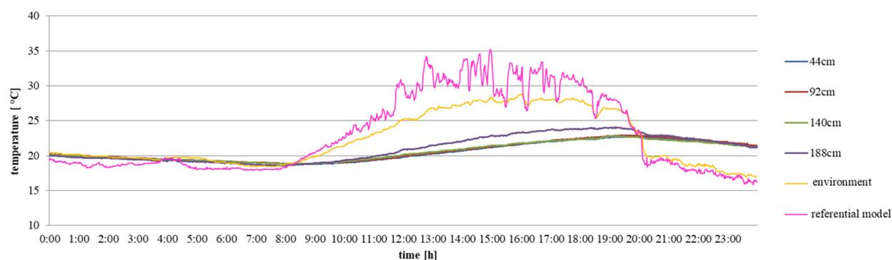
**Fig. 3.** Distribution of temperatures within the substrate on 25 July 2016
