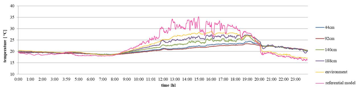
**Fig. 7.** Characteristic temperatures on the wall behind the panel on 25 July 2016
