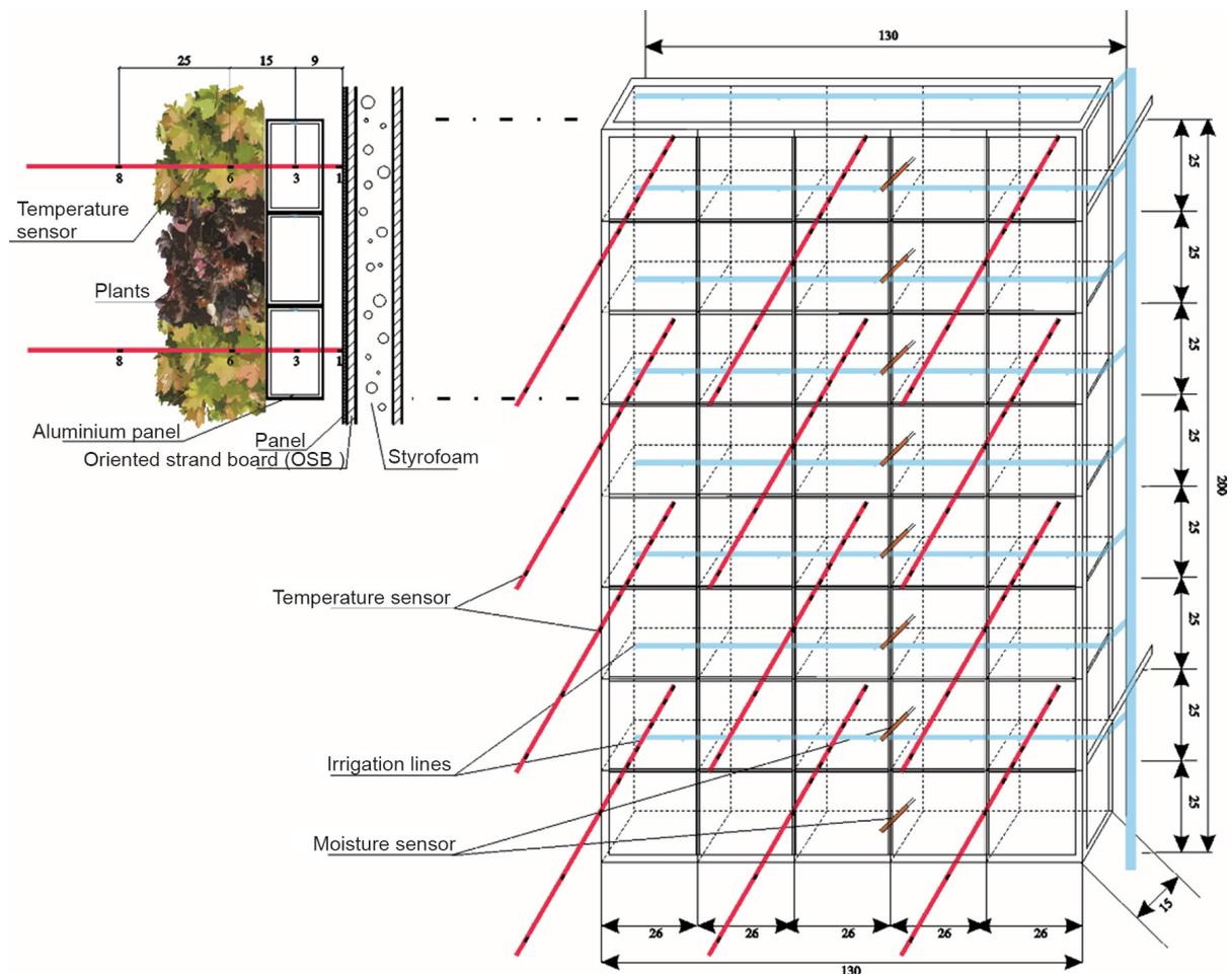
**Fig. 1.** Cross-section diagram of the green wall, along with the location of the sensors
