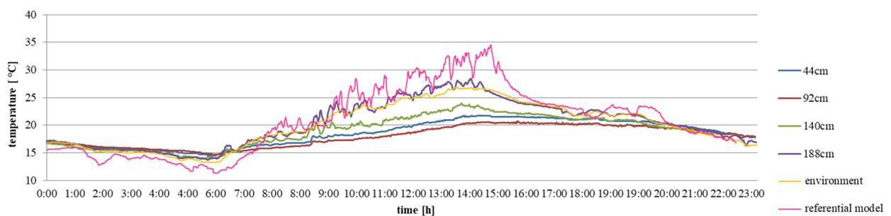
**Fig. 6.** Distribution of temperatures on the wall behind the panel on 28 May 2016
