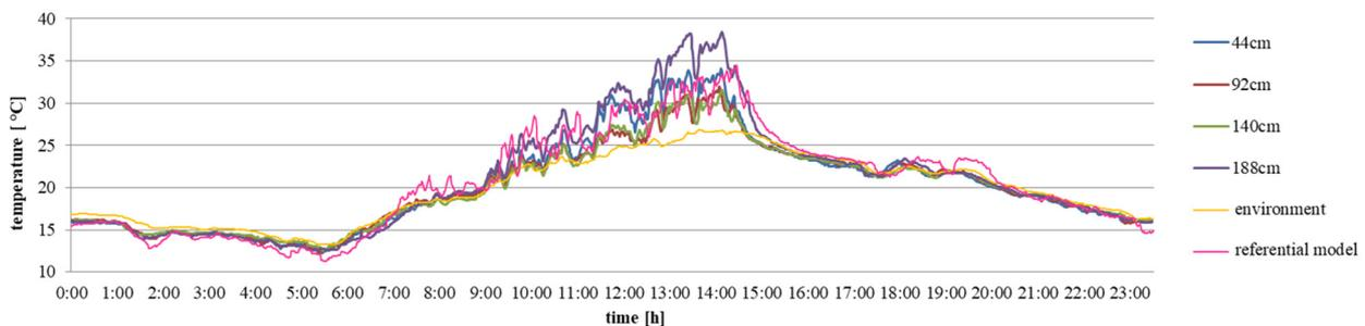
**Fig. 4.** Distribution of temperatures at a distance of 10 cm from the plant surface on 28 May 2016
